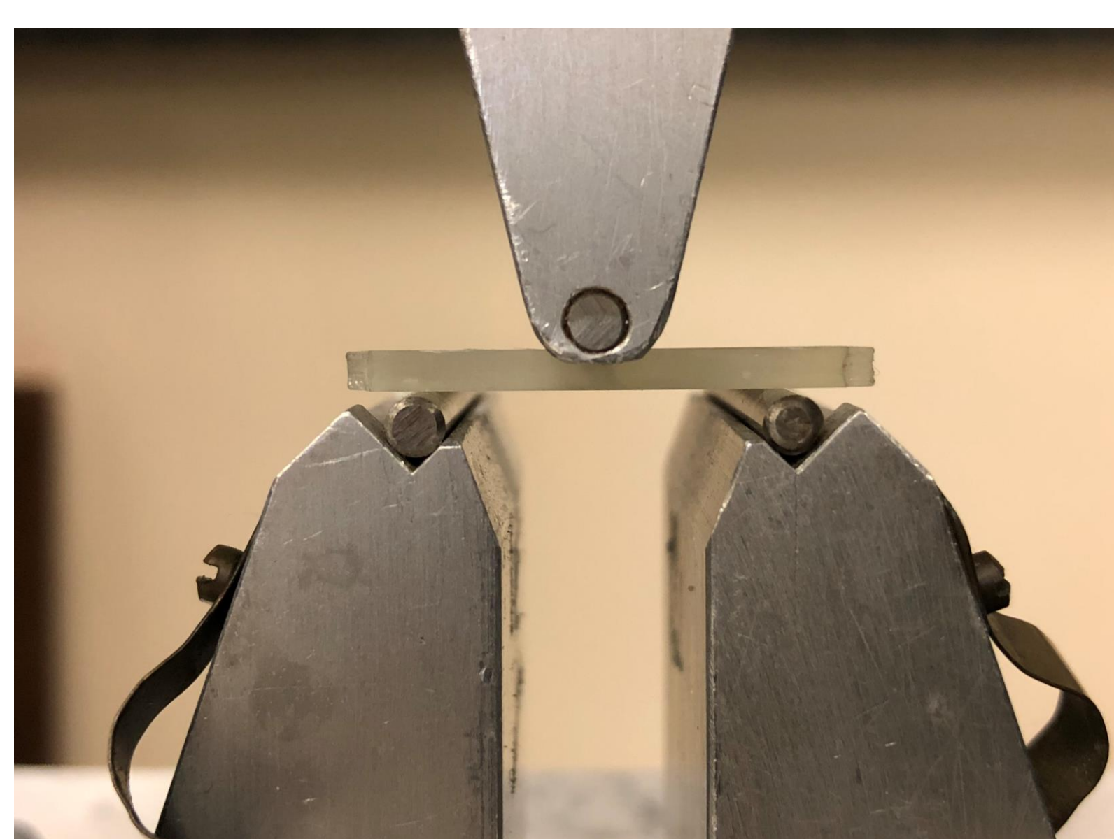
Flexural testing of the splint materials.
